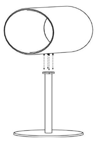
Set the top part in such a way on the mouting plate of the base, that the screws on the bottom of the top part fit into the drillings of the mounting plate. Now screw the nuts in the clockwise direction on the screws and tighten them firmly with a size 10 wrench (metric system).
